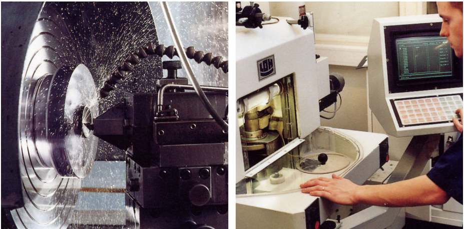
Figure 18.3 LEFT: Diamond turning machine; RIGHT: Lens polishing
